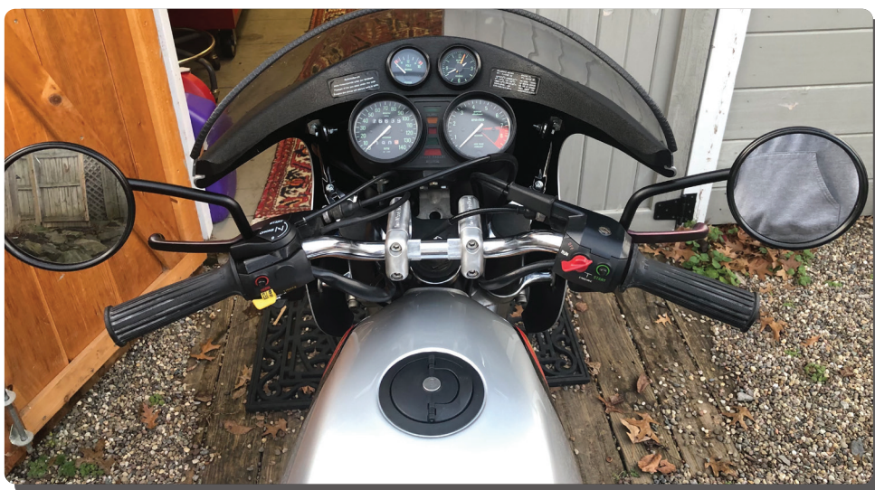
“The following winter included installation of an S-fairing w/instruments, S bars, barbacks, new exhaust system, new seat, new shocks, and crash bars. I rebuilt the carbs, replaced the pushrod seals under the guidance of Oak’s Top End Manual , and installed all the usual bits and upgrades needed on a 38 year old airhead.”
