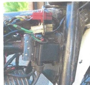
The distance from the box to coils should be min. 10cm
