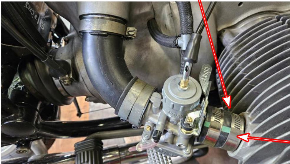
1-1/4" Heater hose from Advance Auto Cut two pices 1-1/2" long part # 28445
