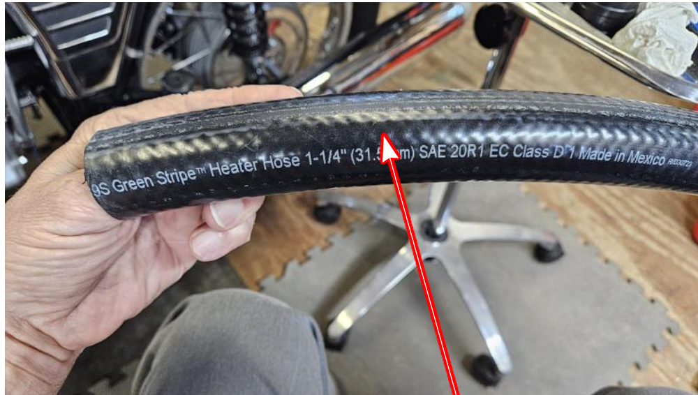
1-1/4" Heater hose from Advance Auto Cut two pices 1-1/2" long part # 28445
